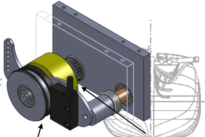
We build our wheel ourselves using a synthetic coating to insure proper traction (this years, we use a shore 30). In addition to our custom wheel, we try to avoid pinion and prefer strap because the backlash is less important, it is cheaper, easy to purchase and easier to use.
